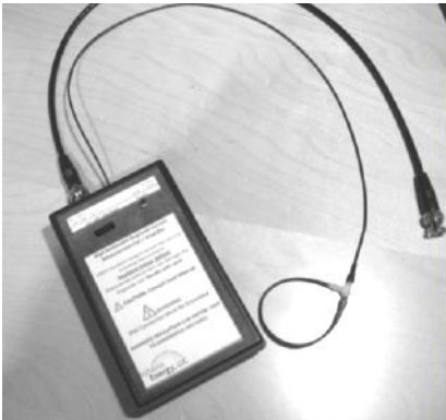
Figure 1. Athena Energy's All-Teflon® Rogowski Coil System
