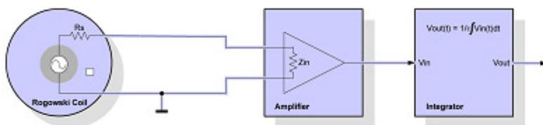
Figure 1: Simplified diagram of Rogowski coil connected to an amplifier and integrator.
