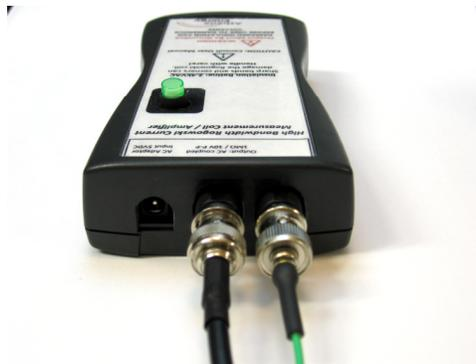
The input power jack is setup for center conductor (+) input with 4-6 VDC supplied. Regulation is provided internally so a simple DC rectified source is all that is necessary.
