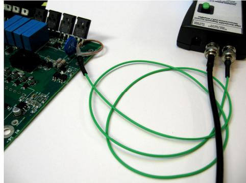
The front of the amplifier box contains the AC adaptor input, BNC Rogowski coil input, and BNC output jack to the oscilloscope.
