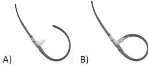
As long as the conductor under measurement is within this coil circle, an accurate current measurement can be carried out.
