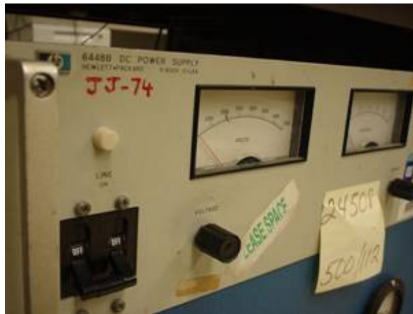
DC Power Supply
